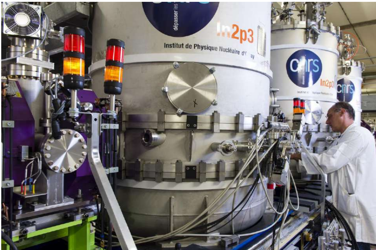
Cryogenic chambers containing the accelerator cavities of the SPIRAL2 linear accelerator at GANIL.
